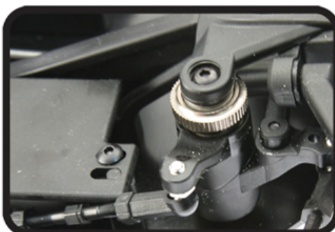
Adjustable top loading servo saver
