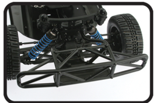
Molded shock absorbing rear bumper
